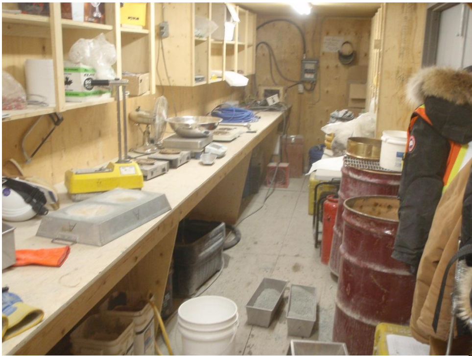
Photo 5: Reconstituting samples in the lab and expediting sieve tests. Some items were moved into the photo for illustrative purposes.
