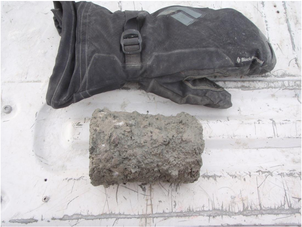
Photo 4: Drilled Core HB12-ND-CORE-DC35-20120214. Some degradation due to spinning gravel.
